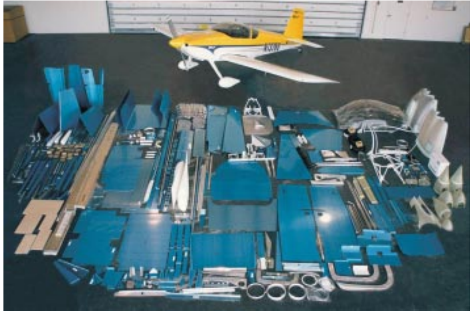
SOME ASSEMBLY REQUIRED. If you're stumped trying to put wheels on your child's bicycle, don't even think about trying this. Laid out on a hangar floor are the parts of a Van's Aircraft kit plane. (Van's Aircraft photo)
